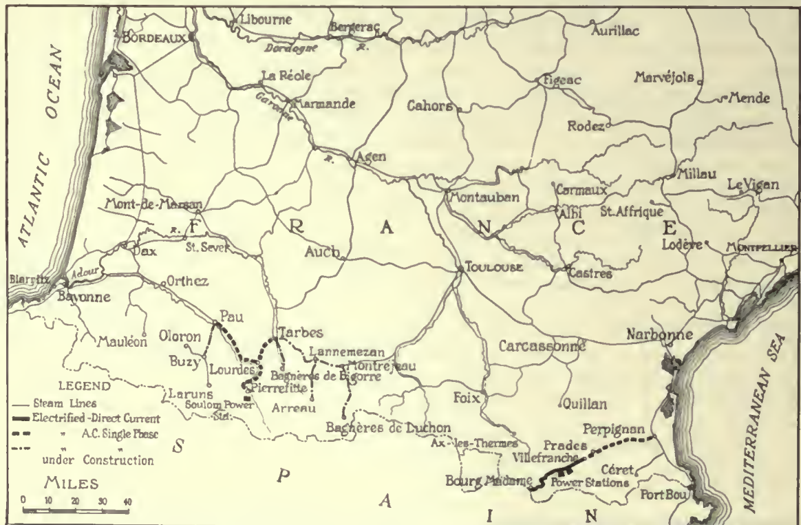
FIG. 468. EASTERN AND WESTERN ELECTRIFIED LINES OF THE MIDI RAILWAY
